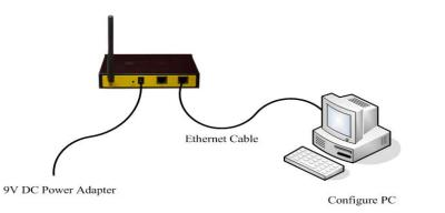
Please modify the IP address of PC as the same network segment address of the router, for instance, 192.168.1.9. Modify the mask code of PC as 255.255.255.0 and set the default gateway of PC as the router's IP address (192.168.1.2).
