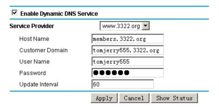
Enable Dynamic DNS Service: Enable DDNS service Service Provider: the DDNS service provider Host Name: The 3322 provider's server hostname Customer Domain: Your custom 3322 domain name. User Name: Your 3322 account username Password: Your 3322 account password Update Interval: The time interval of IP Address update. The "Show Status" button is used to display the current DDNS status.
